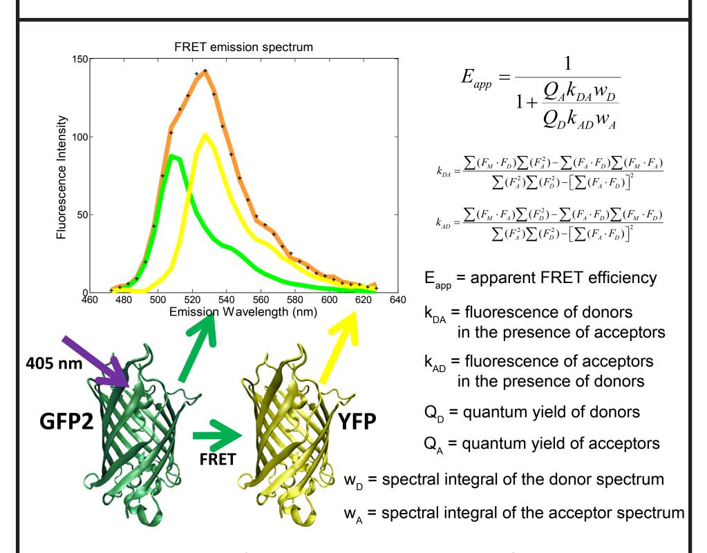
The emission spectra from cells expressing both GFP2- and eYFP-tagged proteins (e.g. orange line above) were unmixed into the donor  $(k_{DA})$  and acceptor  $(k_{AD})$  components (green and yellow lines above). Using the relative strength of the donor and acceptor signal (equation to the right of the plot), we calculated the apparent FRET efficiency (E<sub>app</sub>) for each cell that was imaged.
